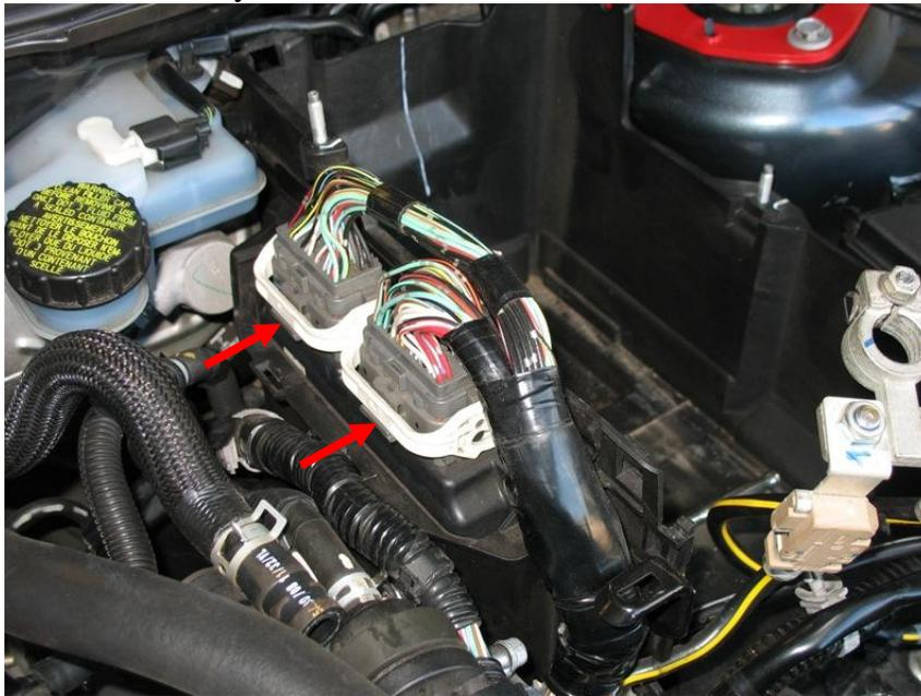
14. Remove the two 10mm nuts securing the wiring harness bracket. Lift the bracket off the studs and lay wiring harness over towards the front driver's side so it's not in your way.
