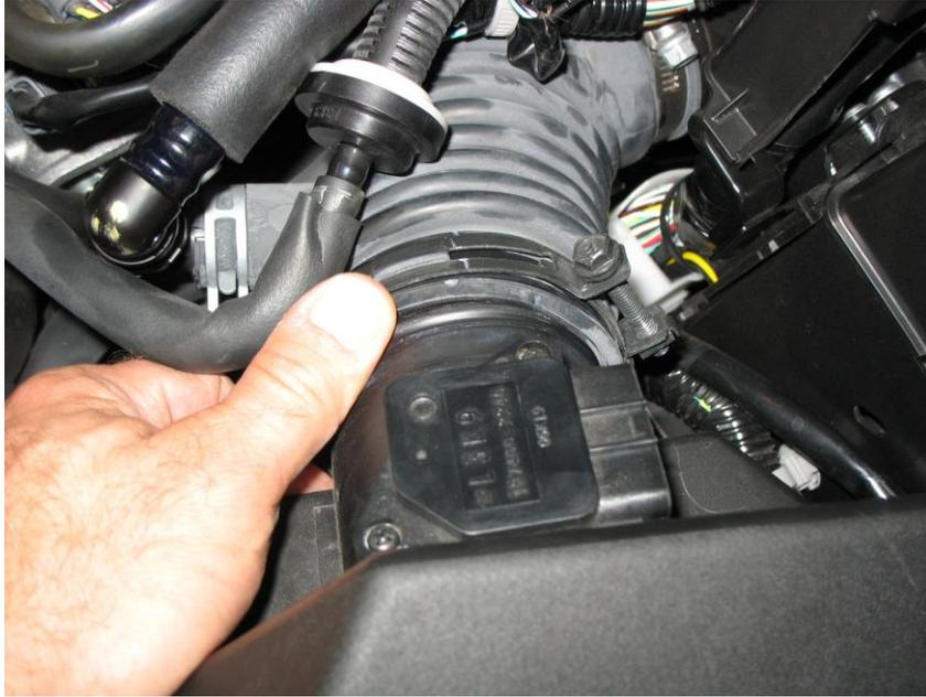
5. Squeeze and remove the clip shown below.
