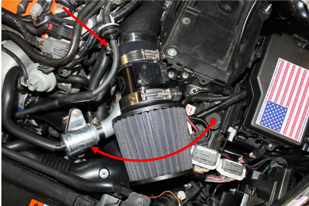
27. If you're installing the 3.5" intake remove the ECU cover, ECU and ECU mounting bracket from the battery box with a philips head screw driver and 10mm socket. Reinstall the OEM battery box and battery.
