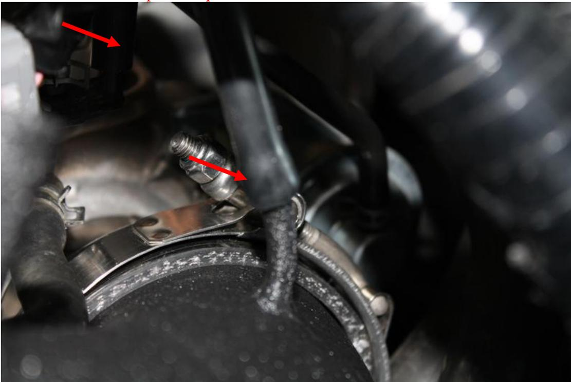
22. Cut approximately 6" off the 5/8" silicone hose included with your kit and install the 90 degree barbed adaptor on to one end. Add the remaining hose to the other leg of the 90 degree barbed adaptor. Install the long hose on to the valve cover vent and the short end on to the intake adjusting the length of the hoses as needed.
