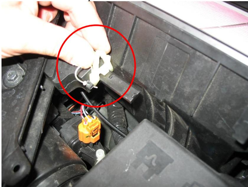
6. Slide the rubber fastener towards the rear of the vehicle.
