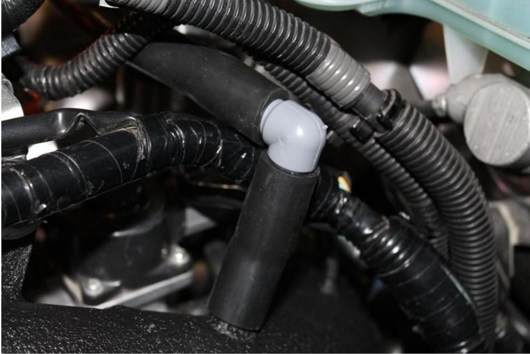
23. Reconnect the bypass hose removed in step 16.
