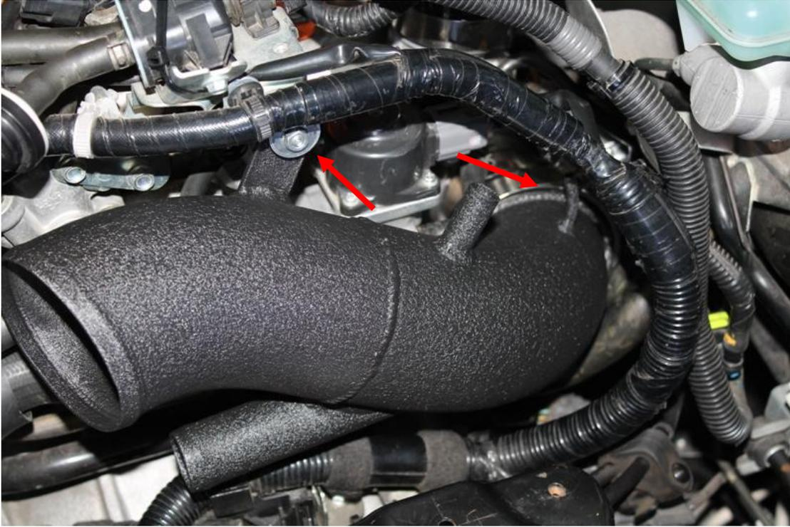
21. Install the included boost control solenoid vacuum line on to the intake and the boost control solenoid.
