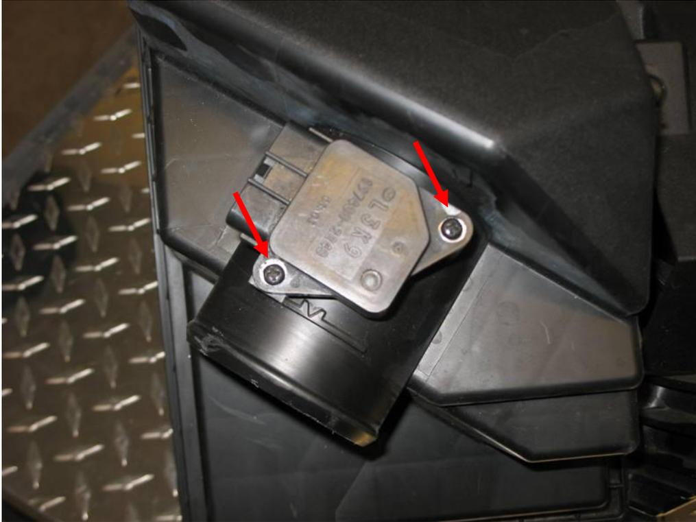
25. Install the MAF sensor using the included screws and tighten with a 3mm allen wrench. Install the JBR Dry Flow Filter and MAF coupler and secure both with the included T-bolt clamps as shown and tighten with a 10mm socket.
