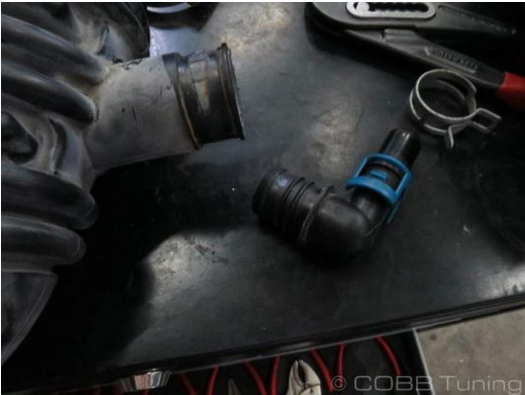
2. Transfer the barbed fitting over to the COBB intake.
