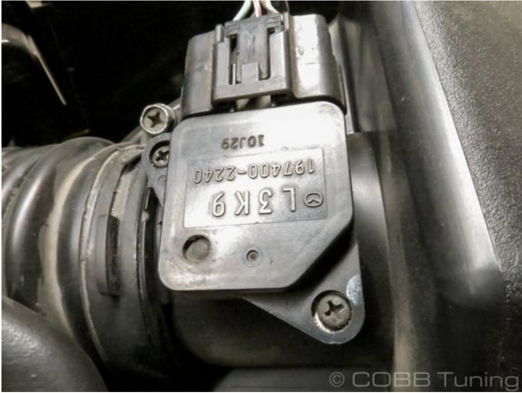
3. Press in the release tab of the MAF connector and unplug the MAF sensor.
